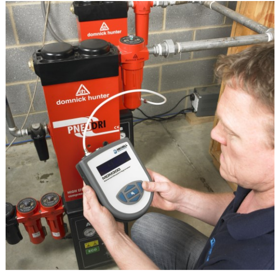
An MDM300 Portable Hygrometer can be used to carry out spot checks on dryers
