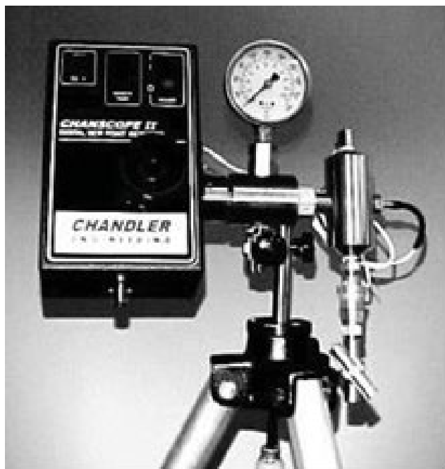
Figure 4 – Bureau of Mines Dew Point Tester 2 Advantages of the Bureau of Mines Device:
