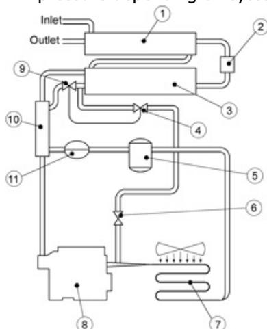
1. Air to air heat exchanger
