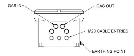
Figure 36 XTC601 Gas Connections and Cable Entries
