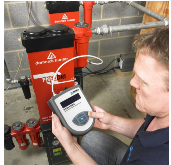
An MDM300 Portable Hygrometer can be used to carry out spot checks on dryers
