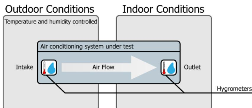
Figure 1. Arrangement of AC system under test
