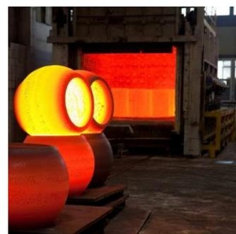
The two types of atmosphere used can be classified as reactive or protective. A protective atmosphere does not interact with the metal being treated and is used to prevent changes happening on the surface of the metal, such as oxidation or decarburization. Reactive atmospheres can be reducing or oxidizing. Reducing atmospheres are most common, made up a mixture of hydrogen and nitrogen. The hydrogen reacts with the metal oxides on the surface of the finished piece, giving a clean finish.
