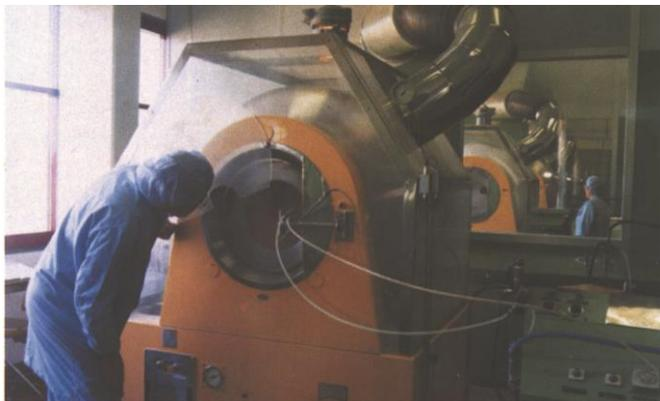
The coating of tablets usually takes place within a perforated rotating drum. There are angle baffles placed in the drum that, along with the air flow inside, help mix the tablet bed. This allows the tablets to be lifted and turned from the peripheries to the centers of the drum to ensure that all surfaces of the tablet is evenly and uniformly coated with the sprayed coating or deposited coating.
