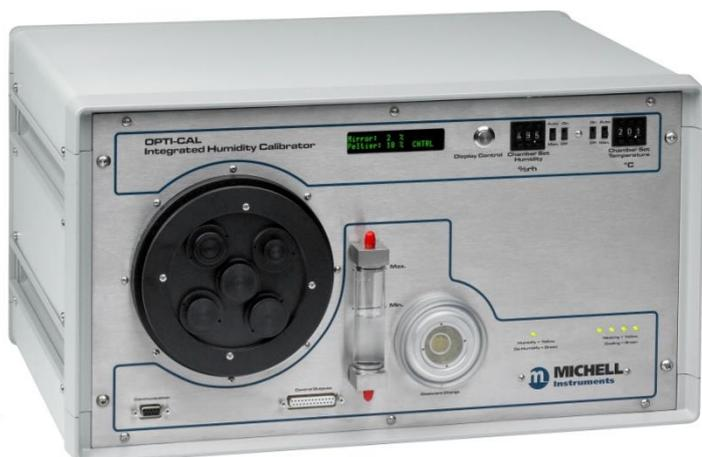
The OptiCal offers all the functionality of the S904, but includes a built-in Optidew Chilled Mirror Hygrometer Reference, which provides fundamental measurement of dew point, and uses this in conjunction with a PT100 to provide a highly accurate measurement of RH. The reference sensor is installed in the rear of the chamber, meaning that useable space inside is not lost in comparison to the S904. This provides the user the facility to carry out traceable calibrations in a transportable package.
